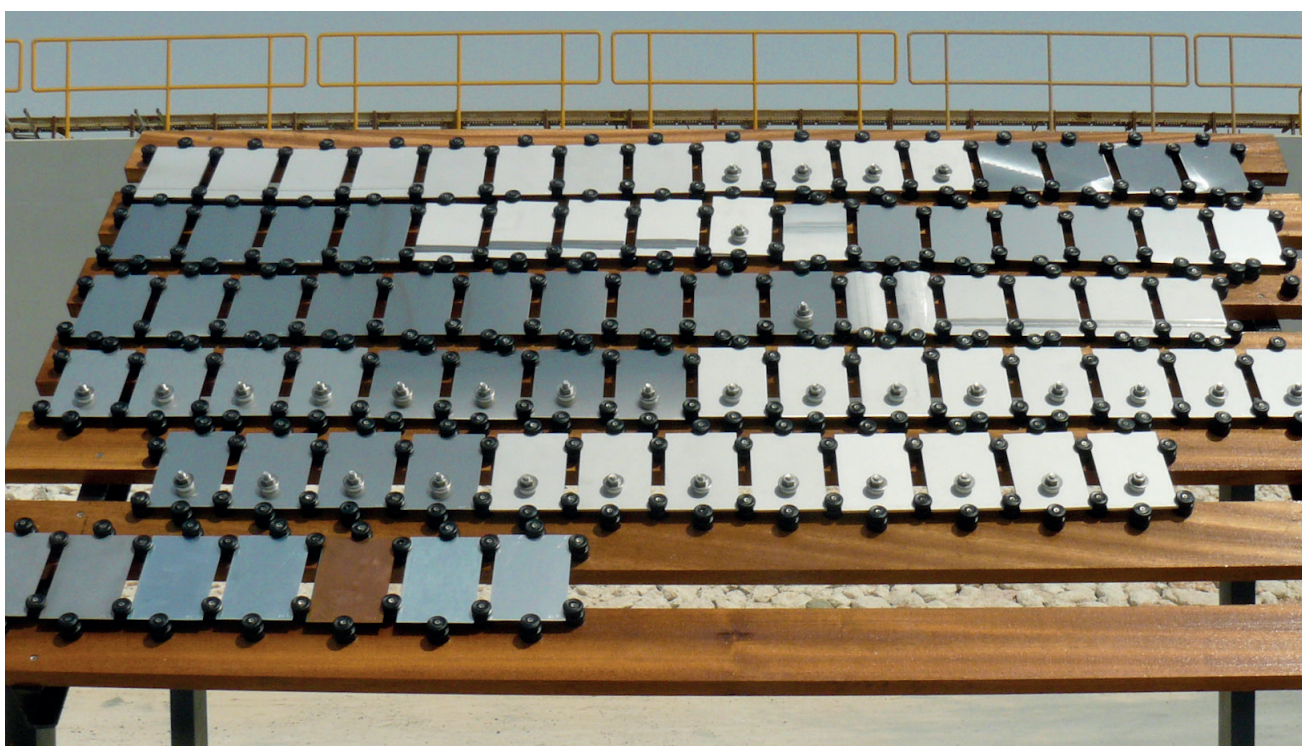
Test rack with samples exposed in open condition at the marine test site in Dubai.
