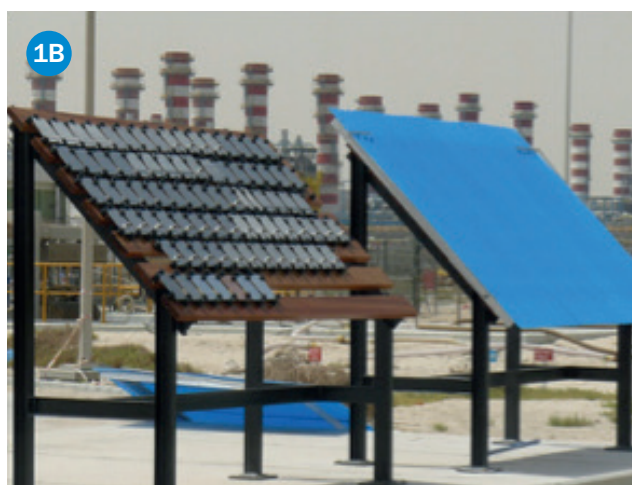
Figure 1 Yellow arrow shows the location where the test samples were exposed at the Dubai Electricity and Water Authority (DEWA) site in Dubai. Reference data is taken from a site within an industrial complex in Jebel Ali [4], marked with a red arrow (1A). Two test racks (open and sheltered condition) with samples for this study (1B–1C).
