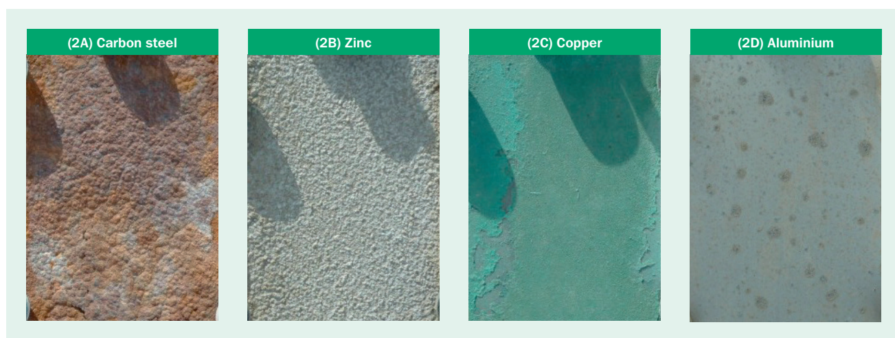
Figure 2 Reference samples to estimate the corrosivity category of the test site. (Note: The diagonal marks are shadows from the specimen holders)
