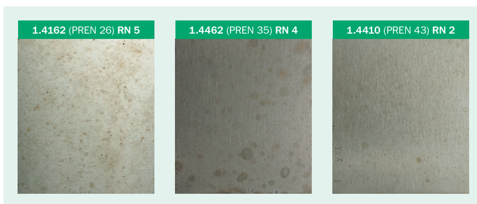
Figure 5 Appearance of duplex stainless steel after four years exposure in open condition
