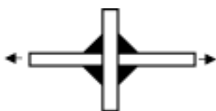
Figure 3b: Geometry and application of load, fatigue design specimen, transverse load carrying fillet weld
