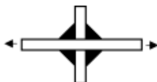
Figure 3d: Geometry and application of load, fatigue design specimen, transverse non-load carrying fillet weld (not used in this investigation, ref. data only)
