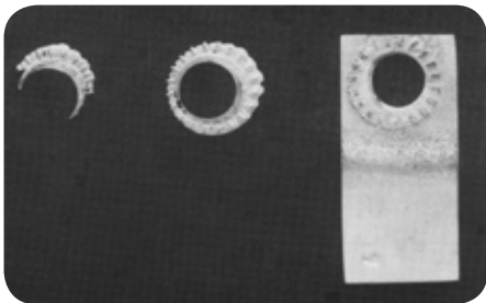
Fig. 17 Titanium specimens exposed in flue gas cleaning systems containing hydrogen fluoride.
