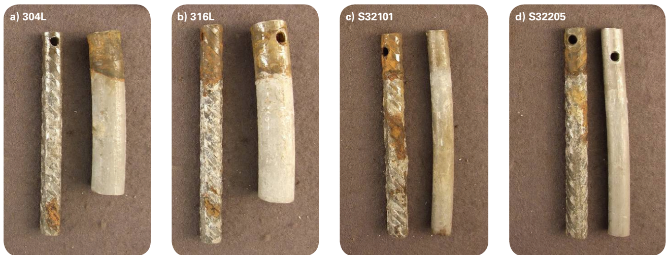
Fig. 2 Uncoupled carbon steels (left) and stainless steels (right) after two years in a concrete block with a) 304L and 2.4% chlorides, b) 316L and 2.6% chlorides, c) S32101 and 2.6% chlorides and d) S32205 3.2% chlorides.
