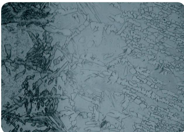
**Fig. 10** Microstructure of weld and S32101 HAZ for a ER2209 plug weld using a shielding gas of 69% Argon / 30% Helium / 1% Nitrogen (mag. = 200X)
