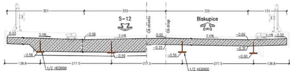
The high degree of prefabrication of the elements translated into shorter assembly times on site. The adopted PreCoBeam solution optimised tonnage (leading to a 30% material reduction), ensured faster delivery times and is expected to decrease maintenance costs. In addition, construction depth was minimised which was particularly important due to site restrictions.
