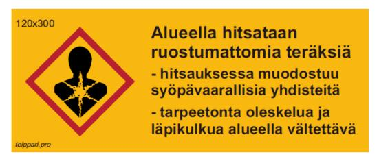
Text in the picture: Stainless steel is welded in this area
