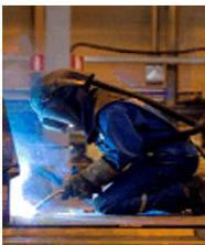
Picture: The correct working method, the blower unit air hose must not be pinched.
