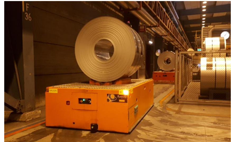
Pictured here is an automated guided vehicle at the cold rolling mill
