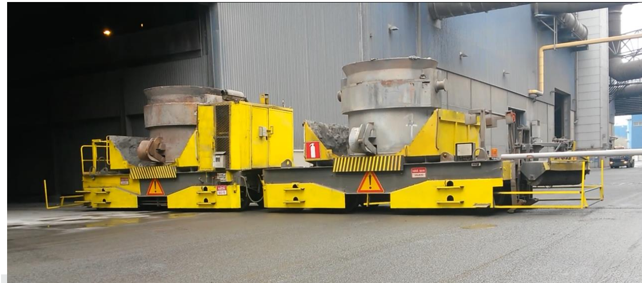
This train carries molten ferrochrome from the ferrochrome plant to the steel melting shop
