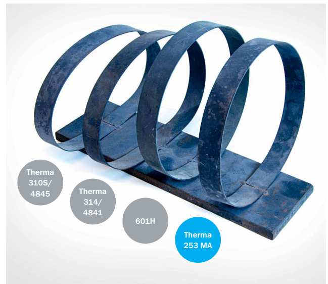
Fig. 3. Therma 310S/4845 and Therma 314/4841 rings collapsed due to their own weight during exposure to 1000°C/1830°F for 35 hours. Sample thickness: 1 mm/0.04 in.
