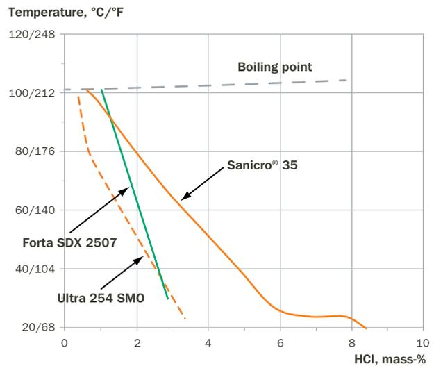
**Fig. 1.** Preliminary isocorrosion diagram for Sanicro® 35 in hydrochloric acid. The line represents a limit, below which the corrosion rate is expected to be lower than 0.1 mm/year. Other grades are included for comparison.
