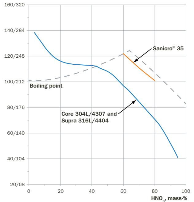
Fig. 3. Preliminary isocorrosion diagram for Sanicro® 35 in nitric acid. The line represents a limit, below which the corrosion rate is expected to be lower than 0.1 mm/year. Other grades are included for comparison.
